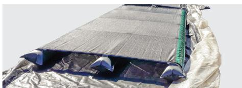
*ADD ON: The GrainPro® Bubble Dryer Bed™ is an inflatable dryer bed that works perfectly with the GrainPro® Bubble Dryer™. It allows high-moisture commodities to be dried at a faster rate. This is possible through the additional airflow created due to the elevated bottom of the bed. It is made of UV-resistant PE mesh supported by pressurized PU tubes.*
