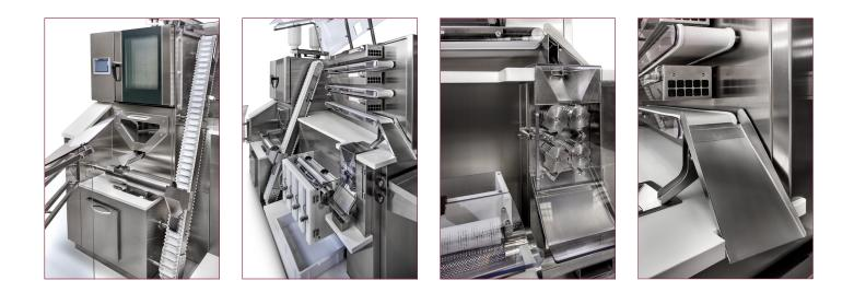
The cocoa then enters the pod splitting unit where the beans are crushed, sieving to 4 different formats and the skin is separated from the nib in the 4 corresponding containers. The nib can be collected into a single container or in 4 different containers.
