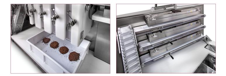
You can obtain the nib in the same cocoa winnowing unit without extraction in the containers. In this case, dust will come out from the first sieve and nibs in different formats in the 3 subsequent ones.
