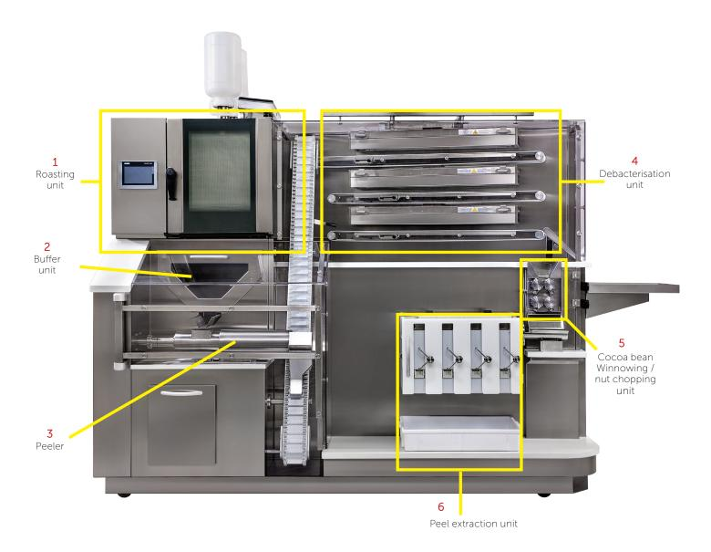
Distributing the product in 4 containers favours the uniformity of the process and makes it possible to vary the amount of cocoa to be treated and, consequently, adapt the machine productivity to ones needs. Different temperatures and times can be set for the two parts of the process.
